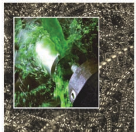
Steel chips: typical stringy, uncontrollable chip formation
