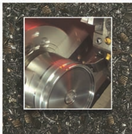
Dura-Bar gray iron chips: fine, compact, consistent and controllable chip formation
