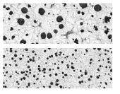
The microstructure consists of Types I & II nodular graphite as defined in ASTM A247. The matrix is 100% ferrite. The edge or rim will have a higher nodular count. Chill carbides will be less than 5% in any field at 100x and will be well dispersed.
