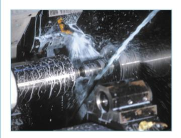
Above: Using continuous cast ductile iron in lieu of some free machining steels can save money by reducing machining cycle times by 25-50%.
