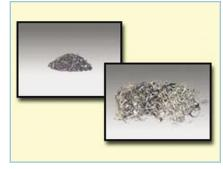
Above: Graphite contained in iron's ferrous metal matrix acts as a chip-breaker which dissipates heat and reduces tool wear.
