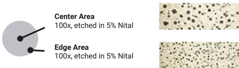
The microstructure consists of Types I & II nodular graphite as defined in ASTM A247. The matrix is 100% ferrite. The edge or rim will have a higher nodular count. Chill carbides will be less than 5% in any field at 100x and will be well dispersed.
