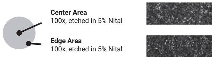
The microstructure will contain Type VII, A, size 4-6 graphite as defined in ASTM A247. The matrix is fully pearlitic. The edge or rim will consist of Type D, size 4-6 graphite in a matrix that is 80% pearlite. Chill carbides will be less than 5% in any field at 100x and are well dispersed.
