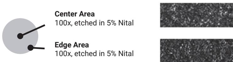
The microstructure will contain Type VII, A, size 4-6 graphite as defined in ASTM A247. The matrix is fully pearlitic. The edge or rim will consist of Type D, size 4-6 graphite in a matrix consisting of 80% pearlite. Chill carbides will be less than 5% in any field at 100x and are well dispersed.
