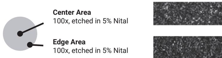
The microstructure will contain Type VII, A, size 4-6 graphite as defined in ASTM A247. The matrix is fully pearlitic. The edge or rim will consist of Type D, size 4-6 graphite in a matrix consisting of 80% pearlite. Chill carbides will be less than 5% in any field at 100x and are well dispersed.
