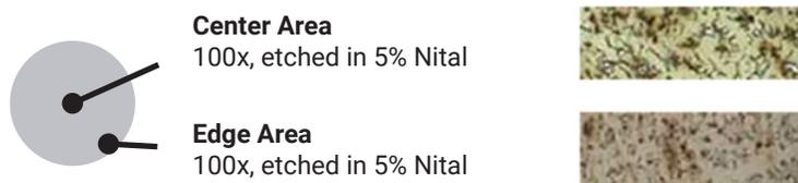
The microstructure will consist of Type VII, A, size 4-6 graphite as defined in ASTM A247. The matrix will be austenite with 5-10% alloy carbide. The edge or rim will contain Type D graphite, size 6-8. Chill carbides are less than 5% in any field at 100x and will be well dispersed.
